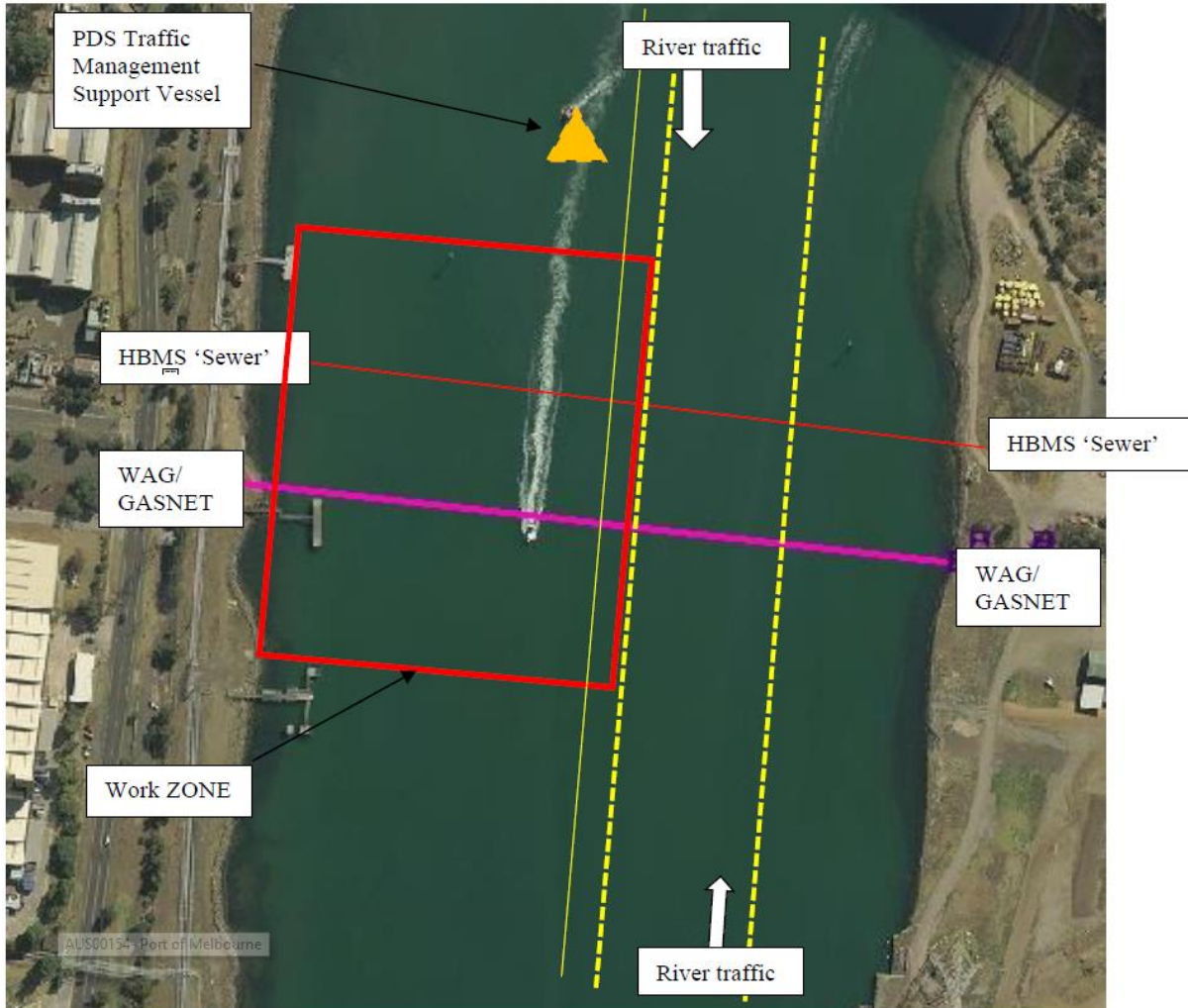
Figure 4. Overview of work zone and general positioning of traffic management vessel – When working WEST of the channel during Closure
