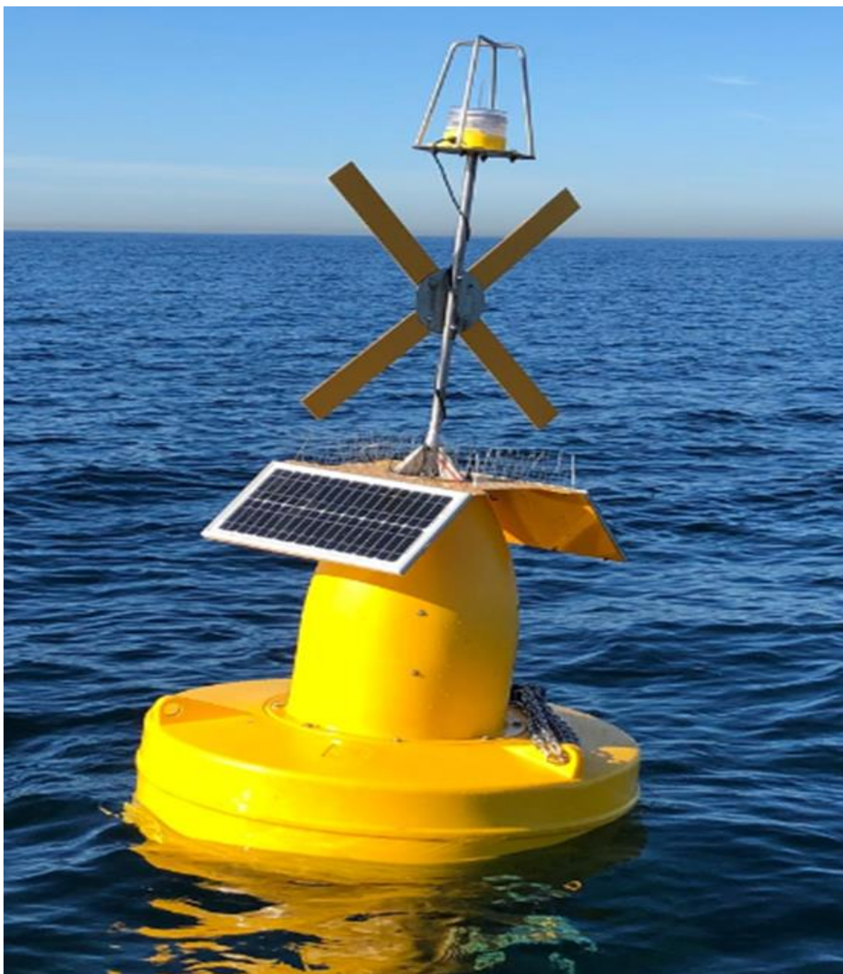
YELLOW MONITORING BUOY WITH SPECIAL MARKER
